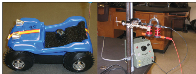
Fig. 2. Modified dune buggy, marble, and electromagnet.
